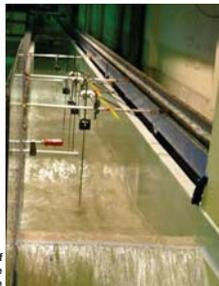
Snapshot of overtopping wave during test in the flume
