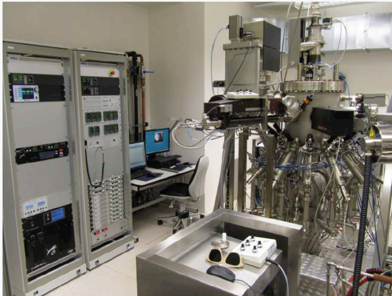
View on the Oxide MBE growth chamber. On the left side: electronic cabinets with power supplies for the effusion cells and e-gun evaporator. In the background: computers for writing recipes for the MBE and for controlling the growth conditions (RGA and RHEED)
