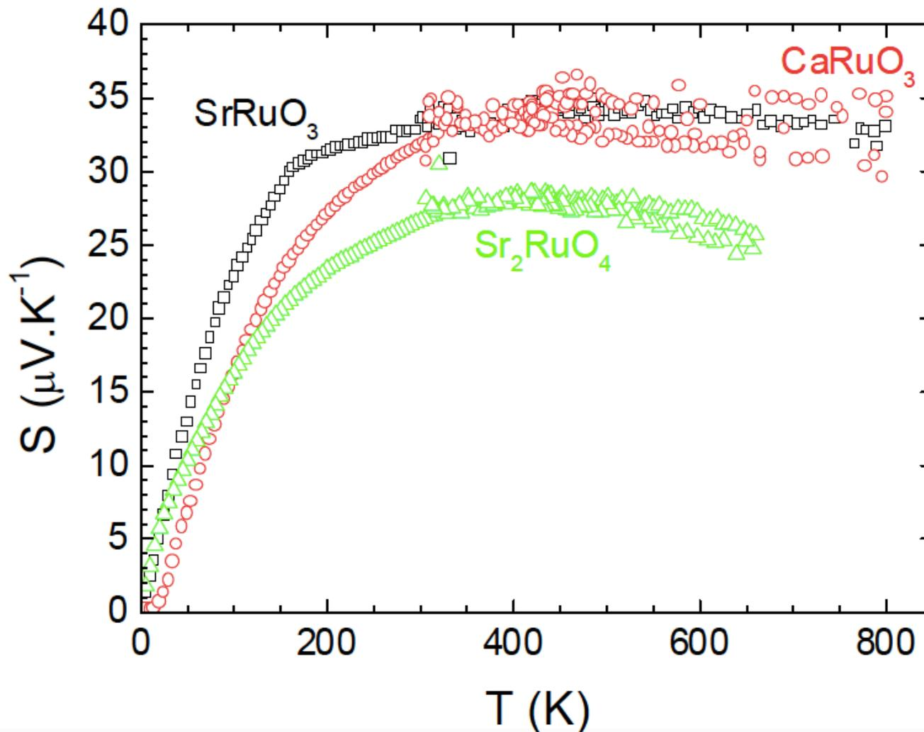
Conspicuous plateau at  $\sim 25\text{-}35\mu\text{V/K}$  around room temperature
