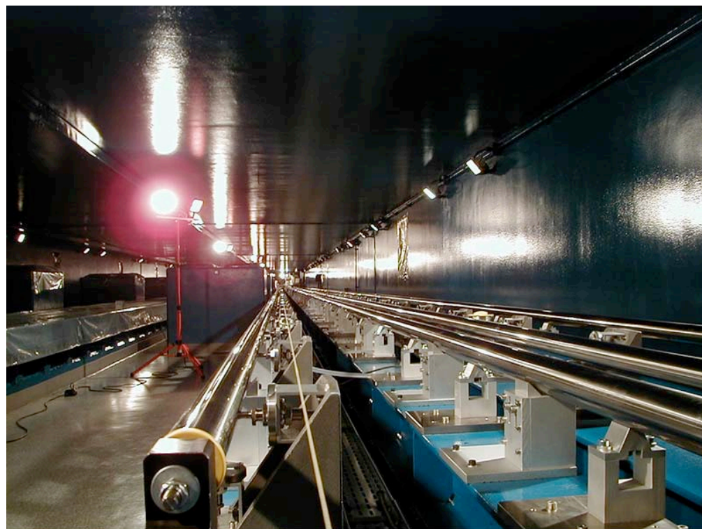
VLTI Delay Lines in the Interferometric Tunnel
