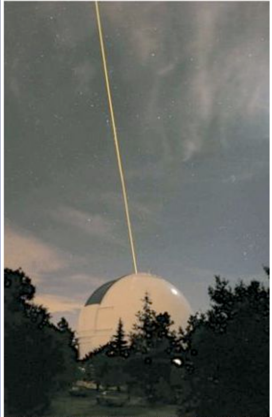
The Lick Observatory Laser Guide Star Adaptive Optics system in operation on July 22, 2003. The
