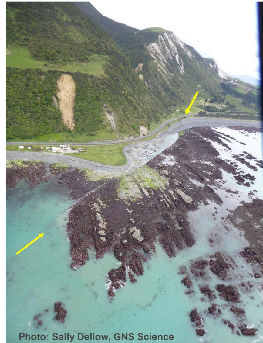
Surface rupture of the Papatea Fault displacing the coastal platform, road, railway and hill country.
