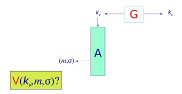
Succe<sup>euf</sup><sub>SG</sub> $(A) = \Pr[(k_s, k_v) \leftarrow G(); (m, \sigma) \leftarrow A(k_v) : V(k_v, m, \sigma) = 1]$  should be negligible.
