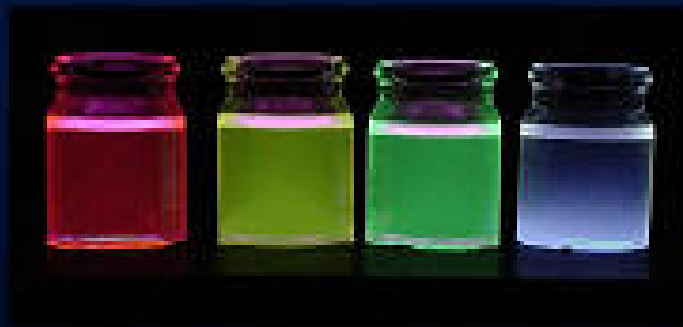
Solutions of differently sized CdSe quantum dots
