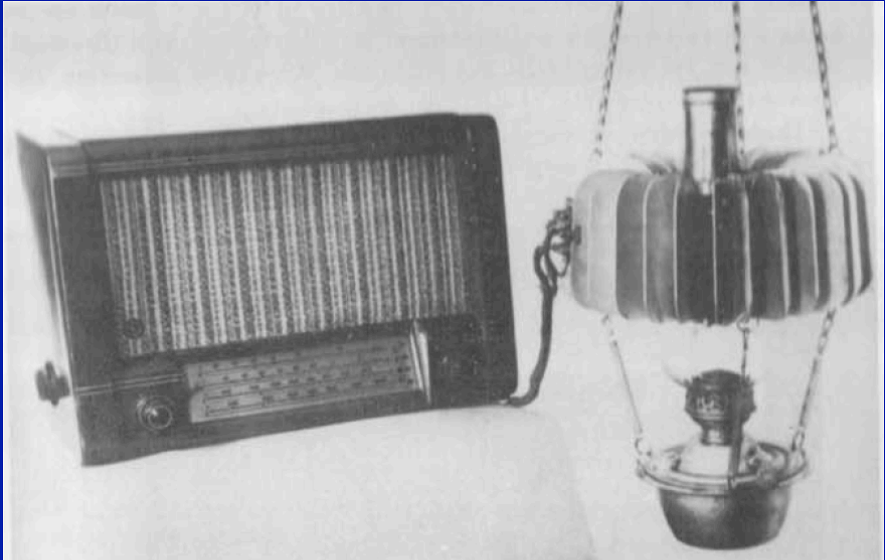
From Abram Ioffe's book: how to operate a few W radio receiver with a kerosene-burning lamp... (USSR, ca. 1955)
