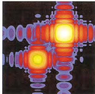
100:1 Star to Planet Ratio Apodization
