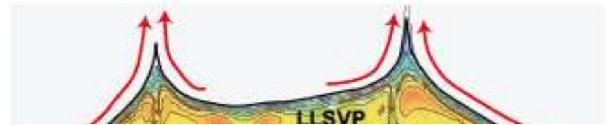
Figure 4. A close-up of the thermochemically dense pile beneath the Pacific Ocean in Figure 3A. (A) A cross-section from the surface to the core-mantle boundary (CMB) displays temperature variations, with the yellow line denoting the boundary of the chemically distinct material in the pile. We identify the thermochemical anomaly as the large low-shear velocity province (LLSVP). Part of the CMB surface is shown in front of the cross-section, along with an isotherm contour (at 0.98, as in Fig. 3). (B) The same cross-section, but only the pile, with a more expanded color scale (colors span T = 0.7 to 1.0). Convective motions are indicated by the arrows. The hottest zones may invoke partial melt of LLSVP material, either at the CMB (denoted as an ultra-low velocity zone [ULVZ] in the figure), or in some isolated locations farther up within the LLSVP.
