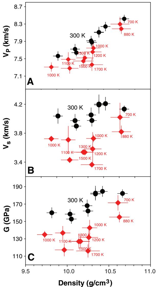
NRIXS measurements on Fe compressed in laser-heated DAC
