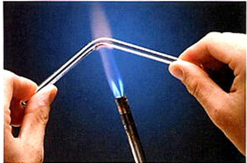
**(B)** A hot glass rod bends and shows ductile behavior without breaking.
