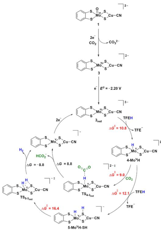
**Figure 7:** Mechanism proposed for the reduction of  $\text{CO}_2$  into formic acid by a dinuclear Mo-Cu complex, mimicking the active site of the CO-dehydrogenase (*Chem. Sci.* **2020**, 11, 5503–5510).
