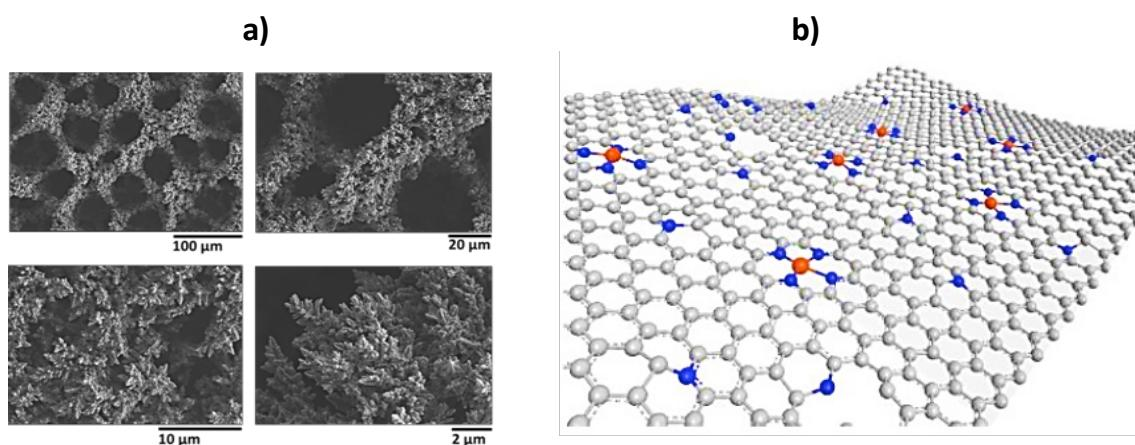
**Figure 4 :** a) Porous dendritic copper-based materials for the reduction of CO<sub>2</sub> into ethylene (*Proc. Natl. Acad. Sci.* **2019**, 116, 9735-9740; *Nature Materials* **2019**, 18, 1222-1227) and the oxidation of water (*Angew. Chem. Int. Ed.*, **2017**, 56, 4792–4796); b) N- and Cu-doped carbon materials, containing Cu single sites, as catalysts for CO<sub>2</sub> reduction to ethanol (*Angew. Chem.* **2019**, 58, 15098-15103).
