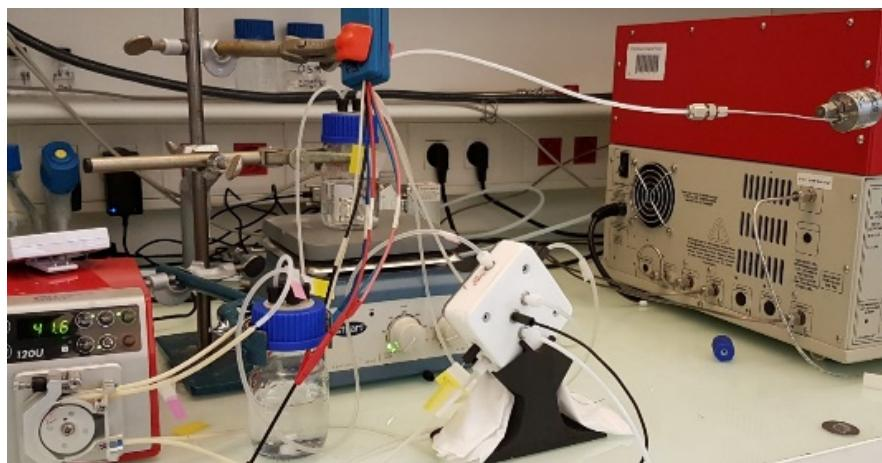
**Figure 8:** Electrochemical flow cell coupled with a chromatograph for the detection of reaction products (*Proc. Natl. Acad. Sci.* **2019**, 116, 9735-9740).
