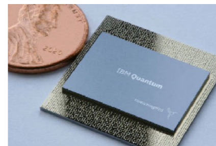
December 2020: An IBM Quantum Hummingbird r2 Processor (65 qubits).
