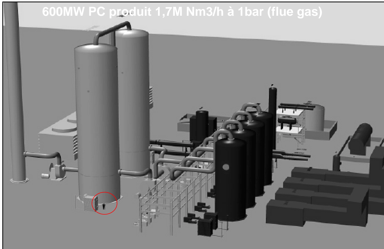
Figure 1: A visualisation of part of the CO 2 Capture Plant - the man standing in front of the two large absorbers gives an impression of scale
