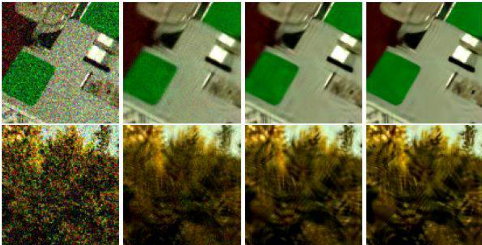
Fig. 3. Artifacts in DDID. From left to right: the noisy image (with \sigma = 30 ), the result of the first, second, and last iteration of the algorithm.
