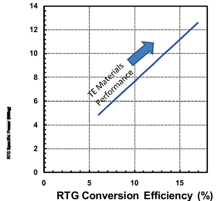
**High efficiency TE materials essential to achieve high specific power and reduce usage of PuO<sub>2</sub>**
