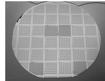
Nextreme (left) thin-film TE cooler and MicroPelt (right) 4”  $\text{Bi}_2\text{Te}_3$  thin-film TE wafer.
