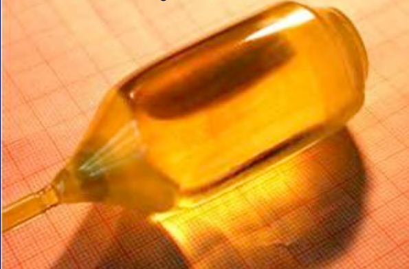
[110] \text{DyScO}_3 , d = 32 \text{ mm}
