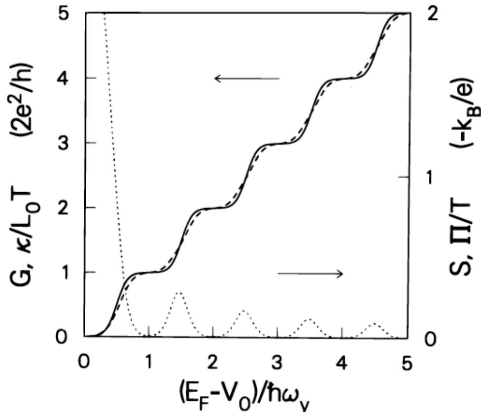
FIG. 3 Calculated conductance  $G$  (full curve), thermal conductance  $\kappa/L_0T$  (broken curve), and the thermopower  $S$  and Peltier coefficient  $\Pi/T = T$  (same dotted curve) for a quantum point contact with a saddle shaped potential, as a function of Fermi energy at 1 K. Parameters used in the calculation are  $\hbar\omega_y = 2$  meV,  $\hbar\omega_x = 0.8$  meV.
