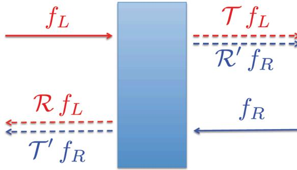
FIG. 1: Transmission and reflection from the scattering region, and probabilities of occupation of a given state.
