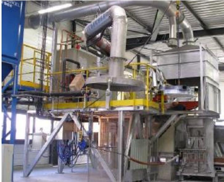
Outside view of the segregation equipment for the production of the upgraded metallurgical silicon
