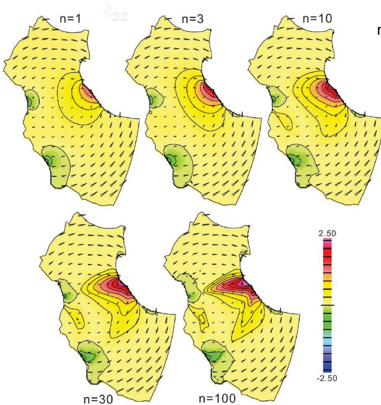
Variation of distribution of modeled vertical strain rate with power-law exponent  $n$ .  $n \sim 30$  best fits the distribution of observed deformation.
