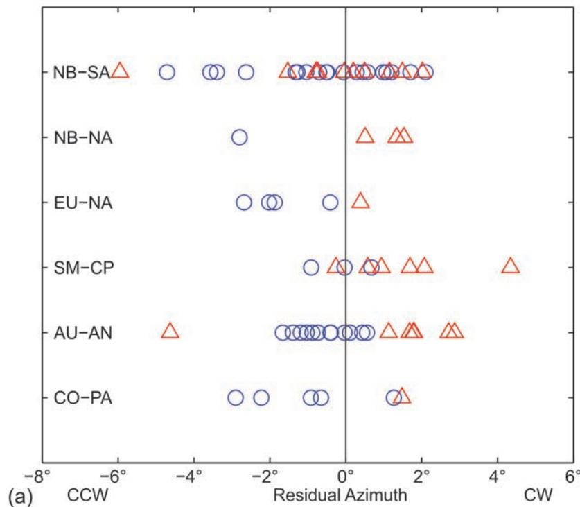
Residuals of transform fault azimuths with respect to best-fitting calculated values for plate boundaries with both **LL (red triangles)** and **RL (blue circles)** slipping transform faults. Rigid plate hypothesis predicts zero difference between RL and LL. Shrinking plate hypothesis predicts that LL tend to be CW of LL. **In 6 out of 6 cases, the mean LL residual is CW of the mean RL residual, consistent with the shrinking plate hypothesis.**
