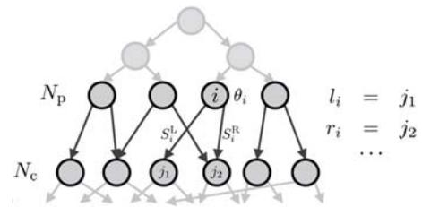
$$E(\underbrace{\{\theta_i\}, \{l_i\}, \{r_i\}}_{\text{features and branches for all parent nodes } i}) = \sum_{\underbrace{j \in N_c}_{\text{sum over child nodes } j}} \overbrace{|S_j|}^{\text{number of examples at } j} \underbrace{H(S_j)}_{\text{entropy of examples that reach child node } j}$$
