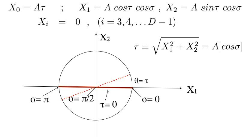
A rigid, rotating rod whose ends move with the speed of light since  $dI/dX_0 = r d\theta / Ad\tau = r/A = |\cos \sigma|$ .
