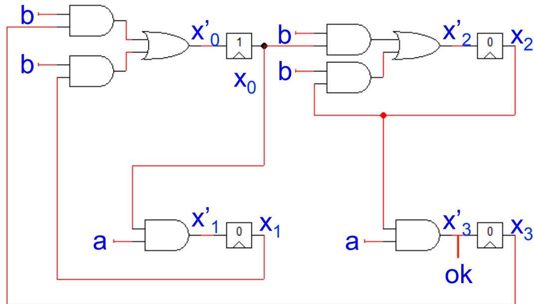
Fonction de transition  $(x'_0, x'_1, x'_2, x'_3) = F(a, b, x_0, x_1, x_2, x_3) =$
