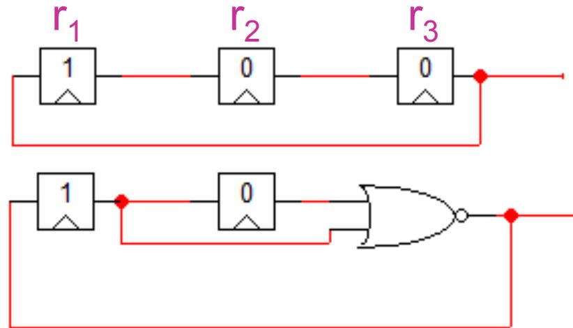
$$A(r_1, r_2, r_3) = r_1 \bar{r}_2 \bar{r}_3 \vee \bar{r}_1 r_2 \bar{r}_3 \vee \bar{r}_1 \bar{r}_2 r_3$$
