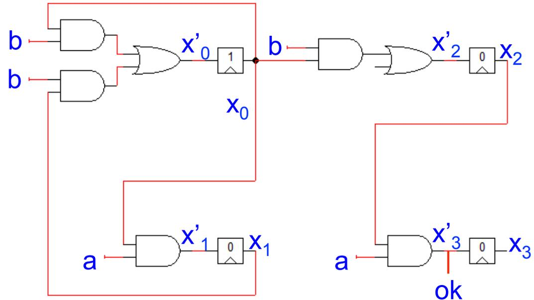
Fonction de transition  $(x'_0, x'_1, x'_2, x'_3) = F(a, b, x_0, x_1, x_2, x_3) = ((e_0 \wedge b) \vee (e_1 \wedge b), (e_0 \wedge a), (e_0 \wedge b), (e_2 \wedge a))$
