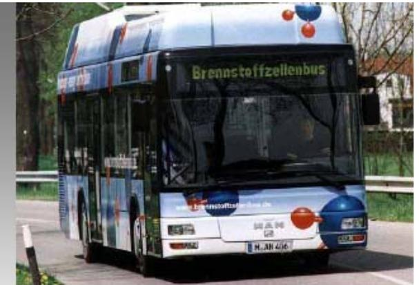
Hydrogen fuelled buses (300 bars) + AFC
