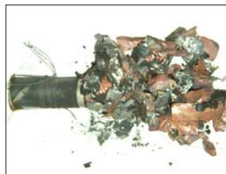
Olivine cells could go to thermal runaway if the cell has high surface area Carbon
