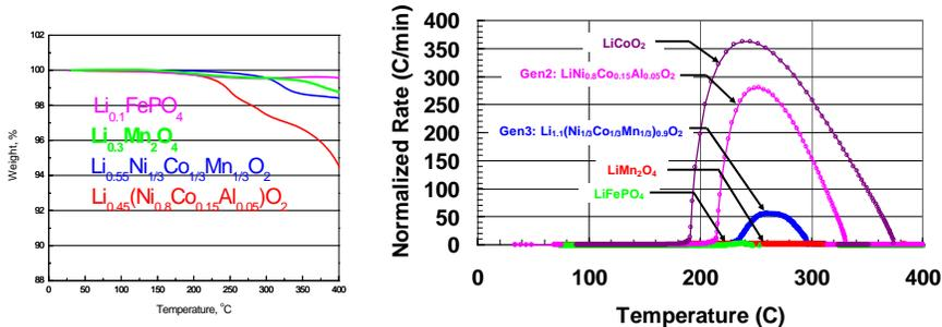
In general the cathode play dominant role in the thermal runaway of the cell. Cathodes that generate less oxygen provide better safety characteristics
