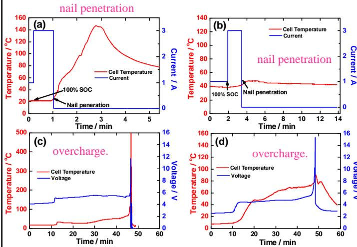
$\text{Li}_{1.06}\text{Mn}_{1.94}\text{O}_4$ /nano- $\text{Li}_4\text{Ti}_5\text{O}_{12}$  shows outstanding safety characteristics both during nail penetration and overcharge.
