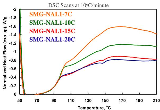
Large particle size and low surface area reduces SEI decomposition heat generation between 80 to 200°C
