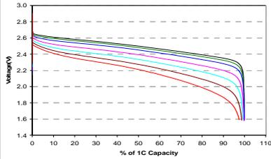
Excellent power LMO/LTO system can discharge within 1 minute
