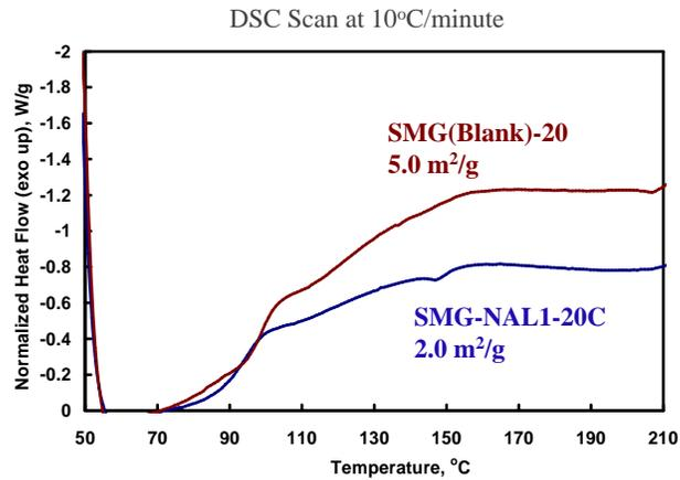
The soft carbon coated material has a lower surface area and exhibits improved thermal behavior between 80 and 200°C
