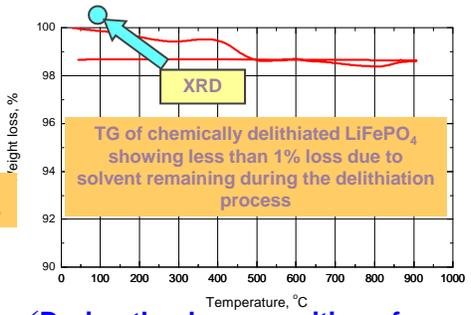
✓ During the decomposition of delithiated  $\text{FePO}_4$ , a new stable  $\text{FePO}_4$  with hexagonal structure is formed
