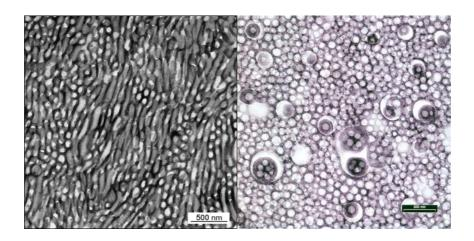
TEM -cuts of two mesoporous silicas obtained from block copolymer templates
