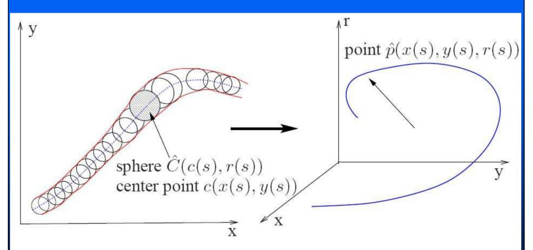
Figure 1. A tubular surface is presented as the envelope of a family of spheres with continuously changing center points and radii. 29/01/2009 21:20 Laurent COHEN, Collège de France, 2009 Examples of 3D Minimal Paths for tubular shapes in 2D Anisotropic Fast Marching algorithm to solve  $\|\nabla \mathcal{U}(x)\|_{\mathcal{M}^{-1}} = \sqrt{\nabla \mathcal{U}(x)^T \mathcal{M}^{-1}(x) \nabla \mathcal{U}(x)} = 1 \text{ and } \mathcal{U}_{p_0}(p_0) = 0$
