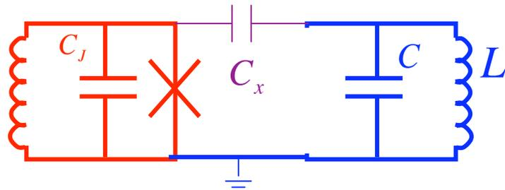
$$H_R = \frac{Q^2}{2C} + \frac{\Phi^2}{2L} \quad ; \quad [Q, \Phi] = i\hbar \quad (3-35)$$
