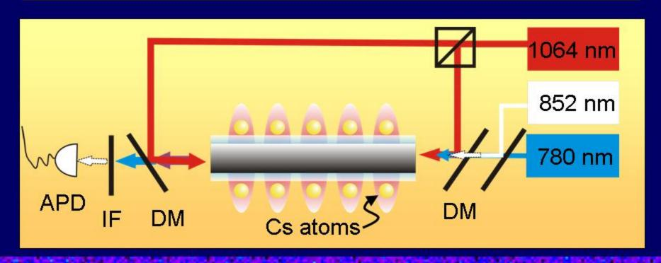
Fluorescence of ~ 2000 atoms trapped 200 nm above fiber!
