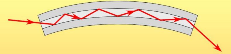
Trick: Narrow down optical fiber until light field gets to the surface.
