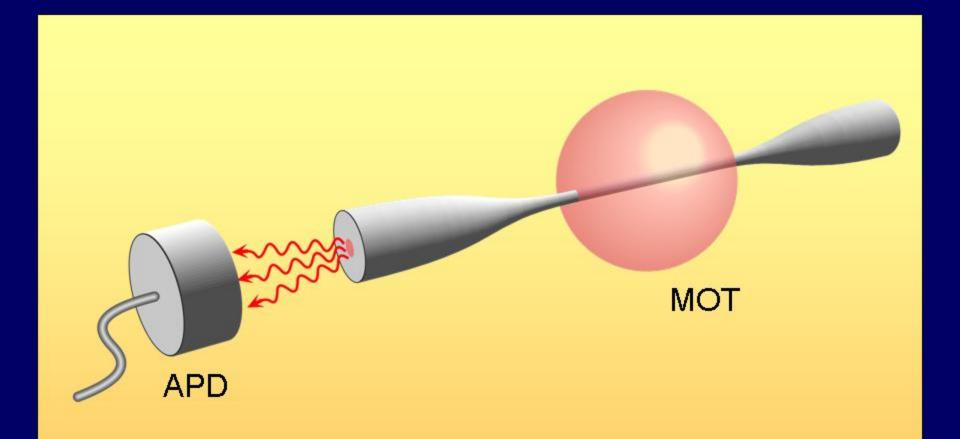
No significant atom loss due to presence of fiber! Very small coupling of MOT laser beams into fiber mode!
