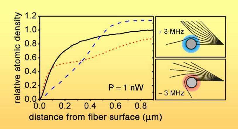
Density close to the fiber is strongly influenced by van der Waals force and light induced dipole forces.
