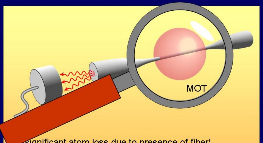
Significant atom loss due to presence of fiber!
