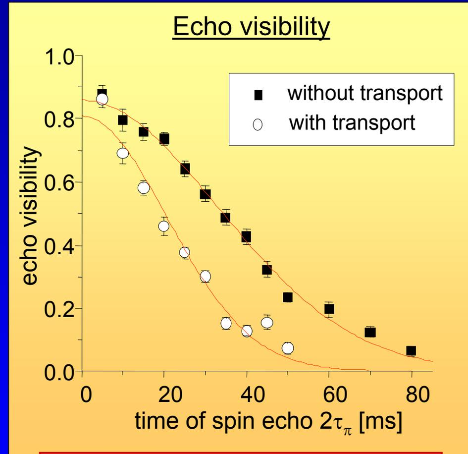
loss of coherence due to heating by abrupt acceleration
