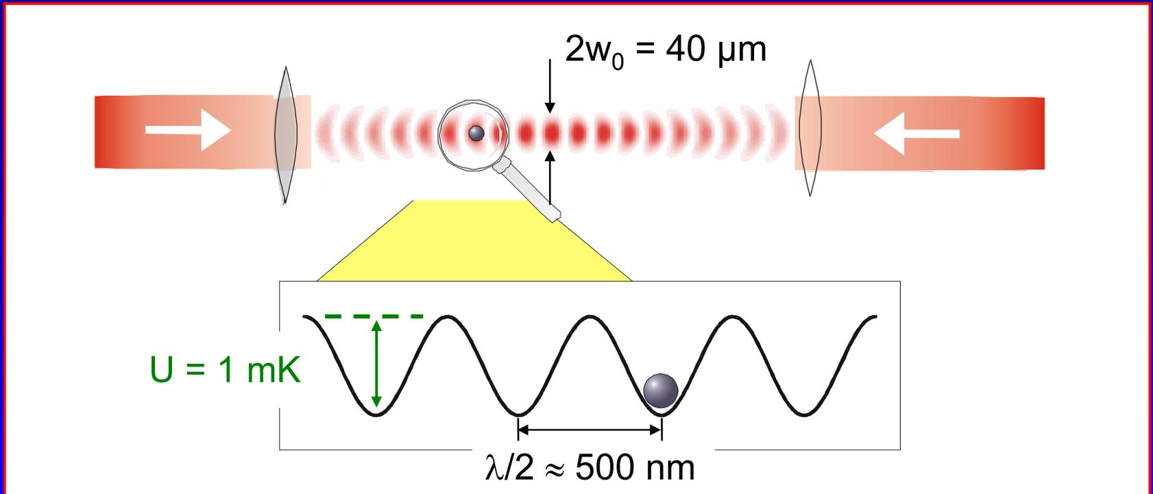
Nd:YAG-Laser ( $\lambda = 1064 \text{ nm}$ ,  $P = 4 \text{ W}$ )
