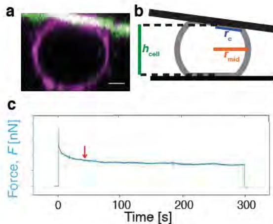
Force exerted on AFM cantilever
