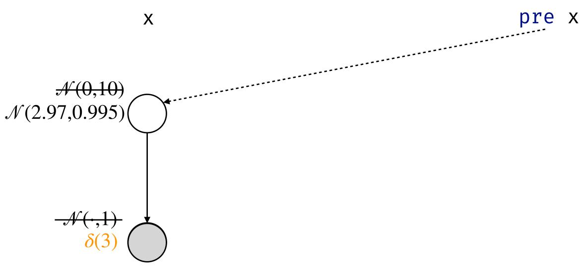
proba tracker (y) = x where rec x = sample (gaussian (0, 10)  $\rightarrow$  gaussian (pre x, 1)) and () = observe (gaussian (x, 1), y)
