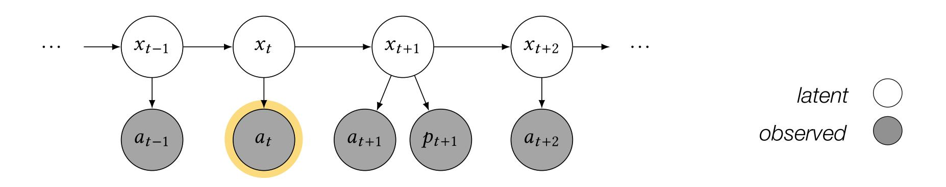
proba tracker (u, acc, gps) = x where  $x = sample (mv_gaussian (motion (u, x0 \rightarrow pre x), noise))$ rec and () = observe (gaussian (get\_acc x, 1.0), acc) and present gps (pos)  $\rightarrow$ do () = observe (gaussian (get\_pos x, 0.01), pos) done
