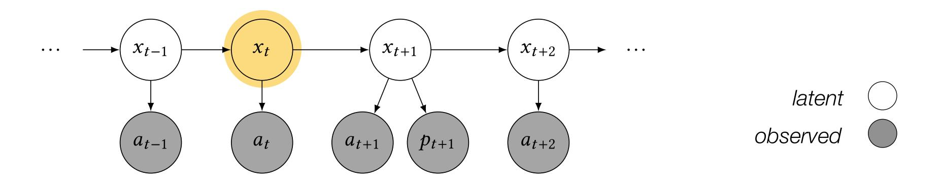
proba tracker (u, acc, gps) = x where rec x = sample ( $mv_gaussian$  (motion ( $u, x0 \rightarrow pre x$ ), noise)) and () = observe (gaussian (get\_acc x, 1.0), acc) and present gps (pos)  $\rightarrow$ do () = observe (gaussian (get\_pos x, 0.01), pos) done
