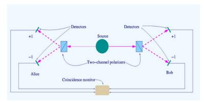
Scheme of a "two-channel" Bell test The source S produces pairs of "photons", sent in opposite directions. Each photon encounters a two-channel polariser with orientation (a or b) to be set by the experimenter. Emerging signals from each channel are detected and coincidences of four types (++, --, +- and -+) counted by the coincidence monitor.
