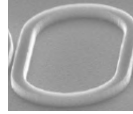
Figure 15. Link connecting two rings in the experiment of Bandres, Wittek, et al. (2018). This link is assumed to be non-resonant.
