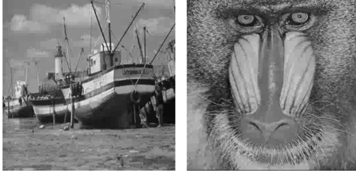
FIGURE 60 – Reconstructed images obtained from quantizing wavelet coefficients with the parameters from Figure 59. The effect of quantization is visible.
