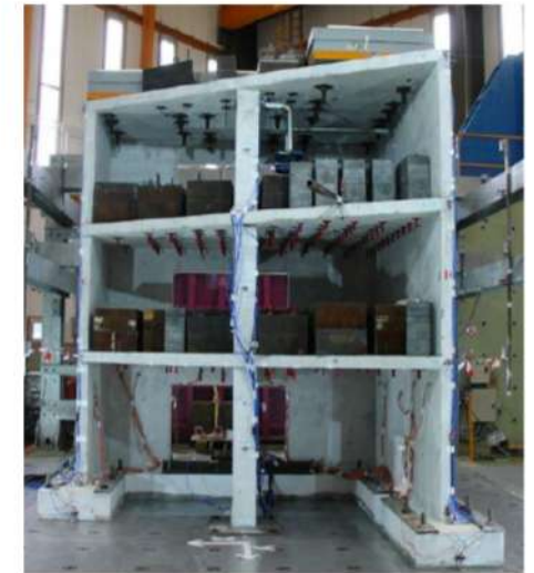
RC specimen of SMART2013 anchored on the AZALEE shaking-table
